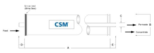
1. Each membrane element supplied with one brine seal, one interconnector (coupler) and four o-rings. 2. All RE2540 elements fit nominal 2.5 inch (63.5 mm) I.D. pressure vessels.
