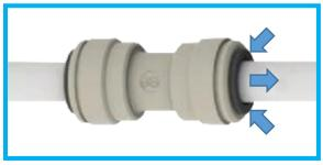
To disconnect, ensure the system is depressurized. Push the collet square against the fitting. With the collet held in this position the tube can be removed.
