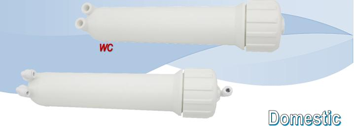
Inlet and outlet ports are moulded directly into the body and cap of the housing via a one piece injection moulding process that requires no solvents or glues during manufacturing.
