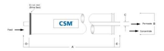
Each membrane element supplied with one brine seal, one interconnector (coupler) and four o-rings.
