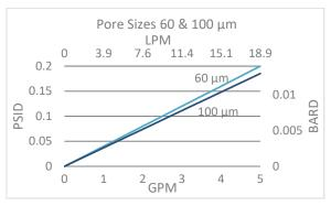
Flow rates for Cartridge filters are per 10-inch length. The test fluid is water at ambient temperature.
