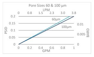
Flow rates for Capsule filters are per square foot of membrane area. The test fluid is water at ambient temperature. Flows are tested using a 2" capsule filter with ½" FNPT inlet and outlet ports. Rates will vary based on end configuration of the capsule.
