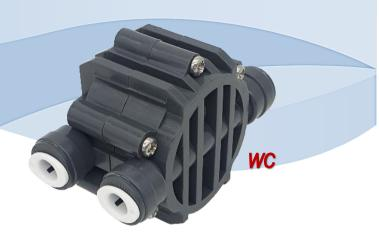
The ASV2000N is a compact valve with four fully integrated 1/4" tubing connections. This valve is designed for a reverse osmosis system. The valve shuts off when the tank pressure reaches 60% of the line or feed water pressure.
